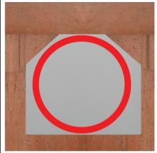
Remove several tiles from the location where Roof Vent will be positioned. You may need to cut some tiles with an angle grinder.
